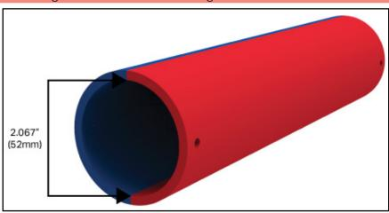
Figure 21: Any vertically expanding parts should be able to fit within a Roller
